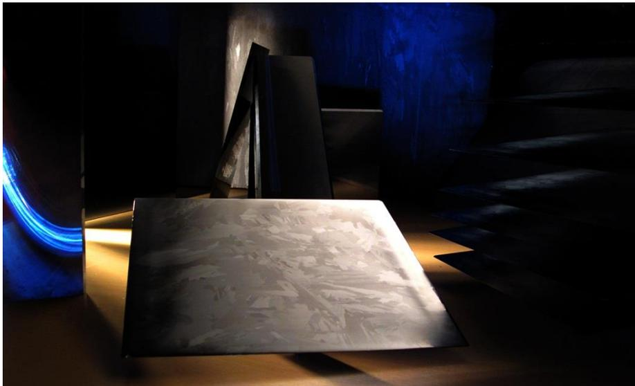
Crystals have applications in a wide variety of fields. Photo of a multicrystalline silicon wafer, which serves as the basis of a solar cell.©Fraunhofer ISE
